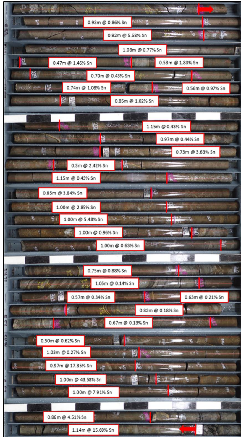
Figure 3: S1671 Drill Core from 224.2m – 252.2m, Showing Sampling Intervals and Tin Assay Results.
